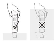
If the display shows ---- indicating the measurement exceeds the range, remove the tester from the sample immediately.  If the HOL d option is enabled in the setup menu, the tester will automatically lock the measurement endpoint and show HOLD icon. Press the Meas key to resume measuring.
